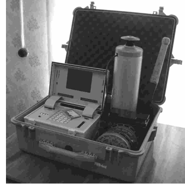
Fig.1 MVC-4DS - portable magnetotelluric station
